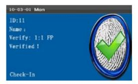
When the system generates a voice announcement "Press FP again!" place the same finger on the fingerprint collector again.
