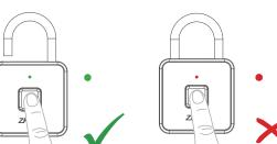
Press a registered finger on the sensor, the green LED lights up if the verification is successful, and then the lock will unlock automatically.
