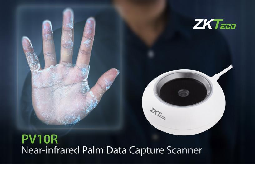
PV10R is a touchless scanner for capturing palm and vein features. It uses a near-infrared fill light, a wide dynamic image sensor, and an aspherical distortion-free camera optical system. It can capture palm and vein images under the palm skin, offering excellent anti-spoofing performance.
