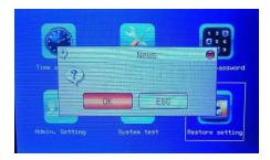
Press the [Confirm] key to confirm and restore the factory settings; when the restore operation is completed, the system settings submenu window is returned automatically. (cancel) key, cancel operation and return to the previous menu interface.
