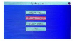
2 · After the SD card test is completed, the "save successfully" prompt box is popped. Press the [confirm] button to close the prompt box
