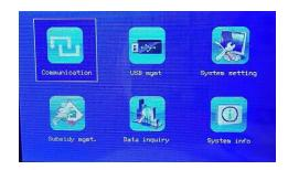
**Communication settings:** Network settings, serial port settings, connection settings, wireless settings and wireless network settings.
