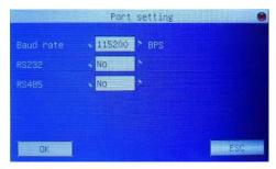
**Baud rate:** the communication rate with PC, has 9600, 9200, 38400, 57600, 115200 these five options. High speed communication is fast, so RS232 communication is recommended. Low speed communication is stable, so RS485 is recommended.
