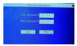
Press the numeric key to enter the 6 bits of the original password; then press the numeric key to enter the 6 bits new password. When you have finished typing the password, press the [Confirm] key to save it. If the old password is typed incorrectly, the screen will prompt you for "password error!" And return to the system settings submenu window.
