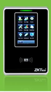
SC700 is a 125 KHz proximity access control terminal incorporated with 3" TFT LCD. The color display and touch screen operation offer a user-friendly and easy menu management.
